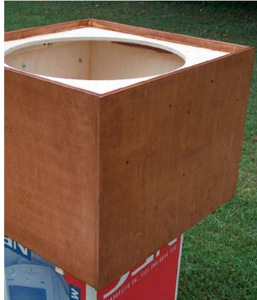
The altitude bearings have traditional cut outs (only window dressing, but Hey! We're going first class, right?) The bearings required several screws to hold them tightly together while they were being laminated (each bearing is a 1.5" plywood sandwich). The screws have been removed, and the screw holes are now being filled. Once the filler is dry, the bearings will be ready for painting black.
