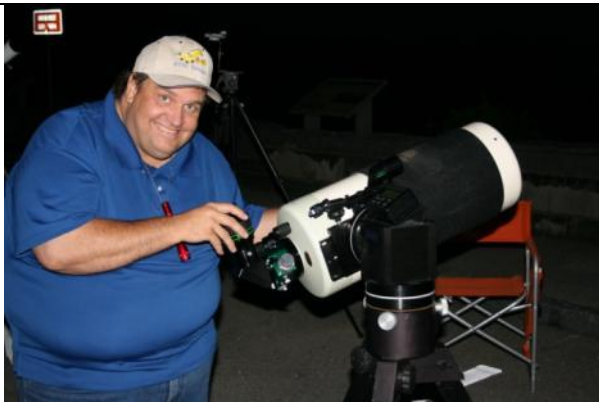
Dennis Hutcheson with his Takahashi Mewlon 210 ( a Dall-Kirkham Cassegrain design 8" scope) on a Discmounts Inc DM-6 (Alt-Azimuth mount) equipped with a Sky Commander XP-4 DSC
