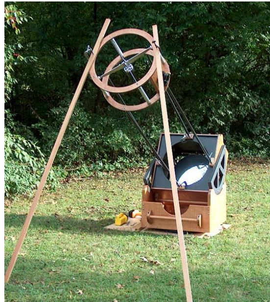
New Sas waits expectantly for nightfall. Note the temporary trusses and bracing.
