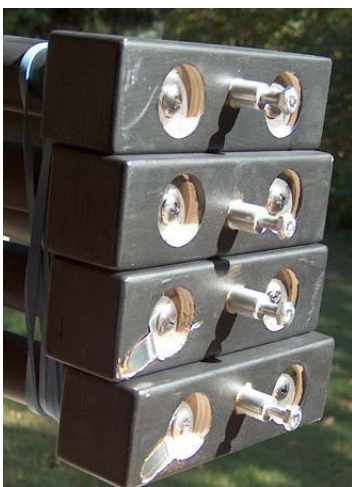
Trusstops and Latchlever – the bolts slide through the aluminum centering posts, and both slide through holes in the lower secondary ring. They are pinned there by the latches. Note the electric contacts recessed in the tops of two of the trusses (they connect the secondary heater to the battery).
