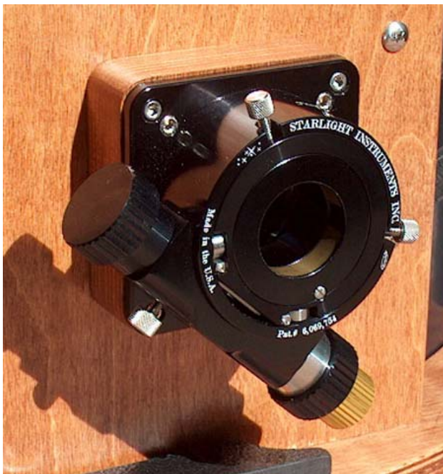
Feathertouch – merely the finest focuser on the market. Note the brass knob on the right: it's for ultrafine focusing, 11:1 reduction gear.
