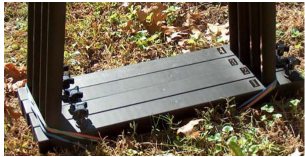
Trussbases – stacked together for transport, you can see their numbers and the star handles that secure them to the mirror box baffle.
