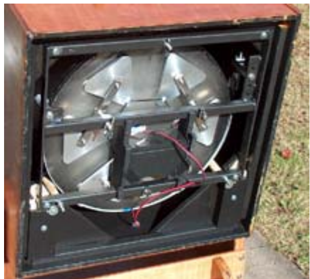
Battery storage box is built into the mirror cell. Instead of dead weight, the battery contributes its weight to the OTA balance.
