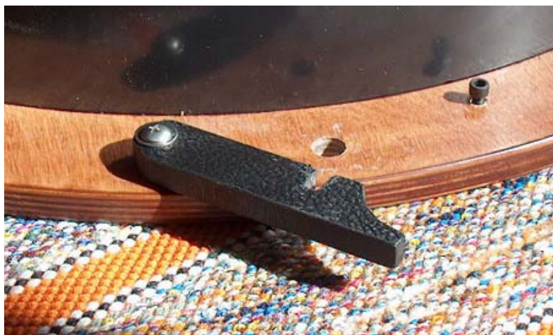
Trusstops and Latchlever – the bolts slide through the aluminum centering posts, and both slide through holes in the lower secondary ring. They are pinned there by the latches. Note the electric contacts recessed in the tops of two of the trusses (they connect the secondary heater to the battery).
