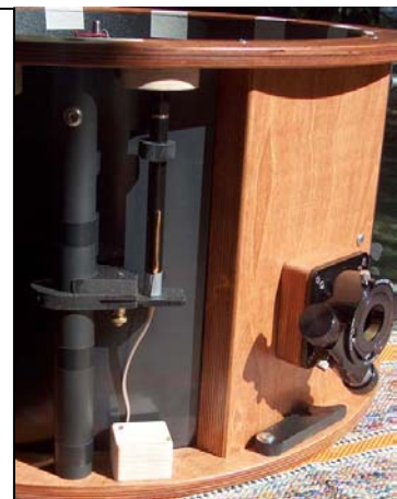
LaserInstalled – that object between the strut and the focuser board is our green laser pointer. Its beam is one mile long and 3 mm in diameter. Slim, eh?
