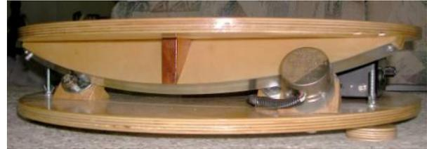
View showing one arc riding on the bearings – the drive motor is on the right
