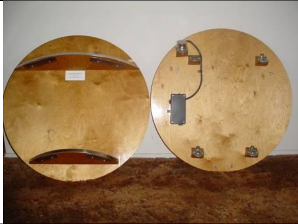
2 arcs on the top half (left disc) and 4 bearing on the bottom half (right disc)
