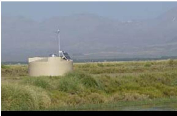
Each detector consists of a plastic water tank measuring 5 feet tall and 12 feet in diameter. When a cosmic ray collides with an air molecule in Earth’s atmosphere, it triggers a shower that multiplies into billions of secondary particles before reaching the ground. When these particles cross from air into water, the speed changes, producing a shock. The shock creates a flash of light that is detected in the dark chamber of the water tank.
