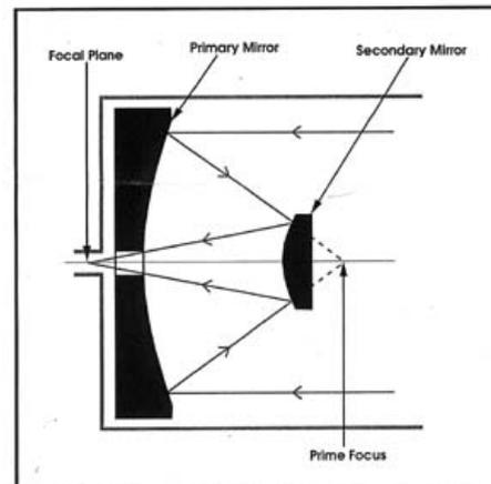
Fig. 1. Invented in 1672, the Cassegrain telescope features a convex hyperbolic surface placed before the focal point of the primary mirror.
