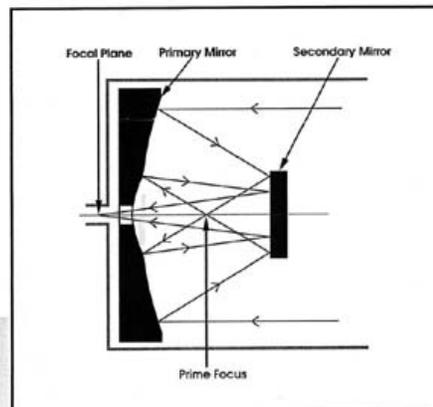
Fig 3. The modified Gregorian design combines the primary and secondary mirrors into a "double mirror" and adds a flat mirror. The length of the telescope is approximately half that of a standard Gregorian, and two-thirds that of a standard Cassegrain.
