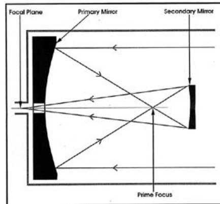
Fig. 2. The earlier Gregorian telescopes features a concave ellipsoidal surface placed behind the focal point, which offer several benefits but requires a much longer tube.
