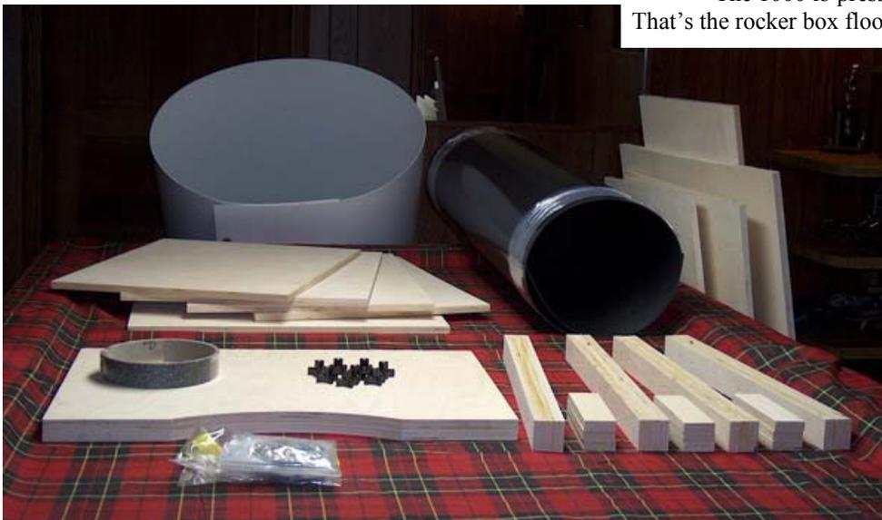
Here are the rest of the parts. Some assembly (and finishing) required. Note the large rolls of black and white 4x8 sheets of ABS and Glassboard. That's the only size they come in.
