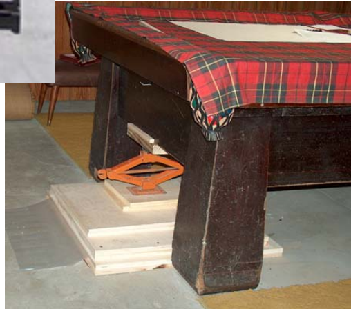
The 1000 lb press in action. That's the rocker box floor getting squeezed.
